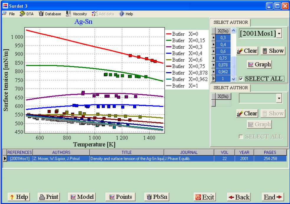
Fig. 6.48. Temperature dependences of surface tensions for liquid Ag-Sn alloy calculated from Butler's model, compared with experimental data
