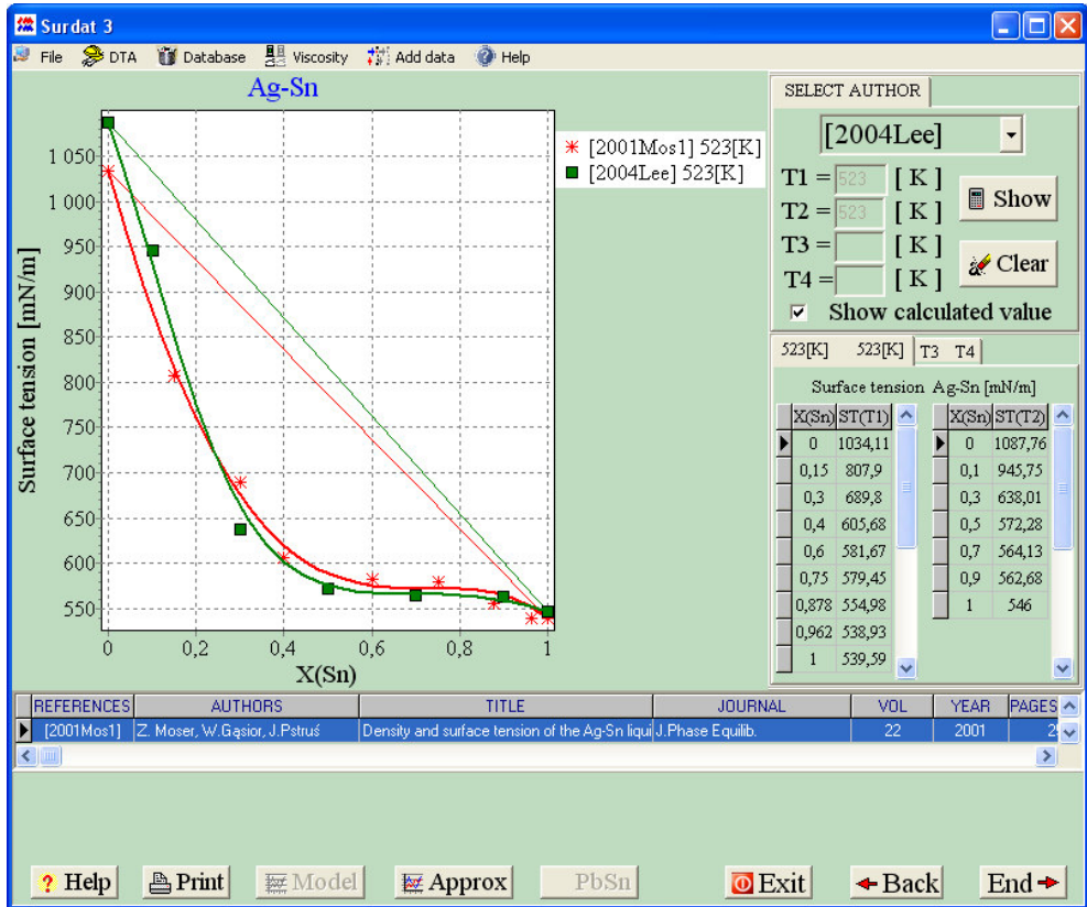
Fig. 6.44. Isotherms of surface tension for Ag-Sn system calculated at 523 K, elaborated by two authors, compared with experimental data
